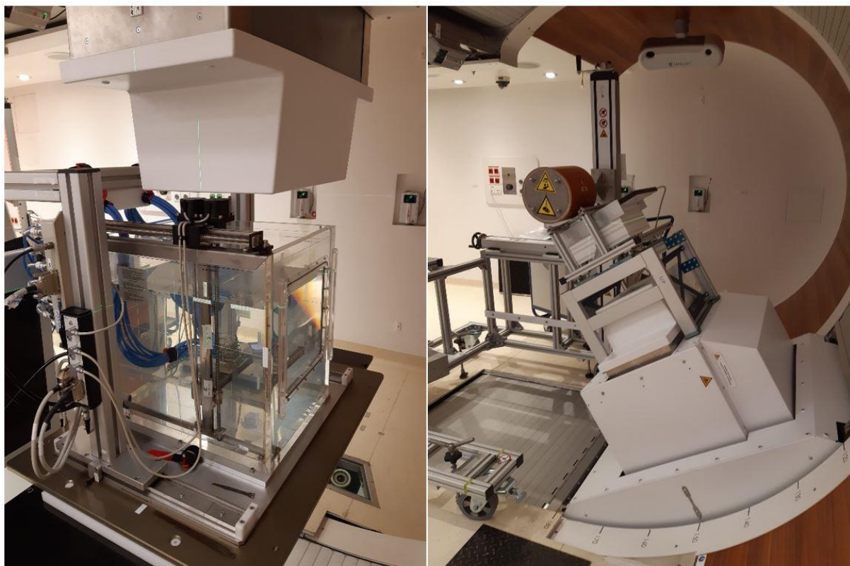
Figure 1: Measurement setup in the gantry room for measurements with the MP3-P waterphantom with PP array-block and with the PTW Octavius in the gantry treatment room
